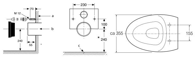
**a.** Finished wall **b.** WC-connection **c.** Finished floor \*Sitting height: 400-450 mm above the floor
