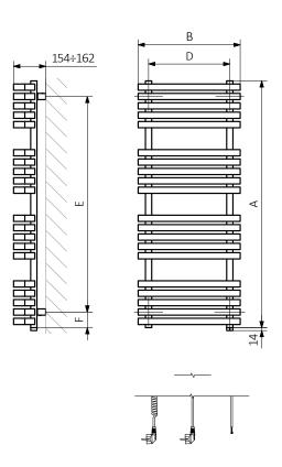
$A-Height\ B-Width\ C1-C5-Distance\ between\ pipe\ centres\ D-Horizontal\ distance\ between\ mounting\ bracket\ centres\ E-Vertical\ distance\ between\ mounting\ bracket\ F-Distance\ between\ a\ mounting\ bracket\ and\ the\ bottom\ of\ the\ radiator$
